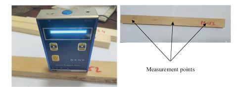
Figure 4 Measurement of roughness on samples Slika 4. Mjerenje hrapavosti na uzorcima
