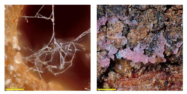
**Figure 5** Secondary, clamp fungal mycelium in oak wood vessel (A) and slime fungus growing on wood surface (B) **Slika 5.** Sekundarni micelij stezaljke u traheidi hrastovine (A) i sluzava gljiva koja raste na površini drva (B)
