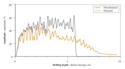
**Figure 8** Resistograph profiles of non-decayed and decayed beam in the analysed mill **Slika 8.** Profili rezistografa neraspadnute i raspadnute grede u analiziranome mlinu
