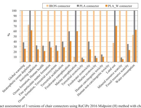
Figure 5 Impact assessment of 3 versions of chair connectors using ReCiPe 2016 Midpoint (H) method with characterization of results, excluding long-term emissions
