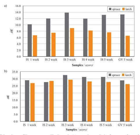
Figure 6 Colour change of Norway spruce and larch samples (a) exposed to weathering from one to five weeks (b) after weathering and treatment with iron (II) sulphate (IS) and green vitriol GV)
