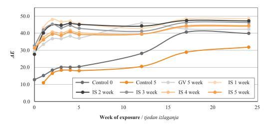
**Figure 7** Colour change ( $\Delta E^*$ ) of control and iron (II) sulphate and green vitriol treated Norway spruce wood samples, exposed outdoor at 45° to south
