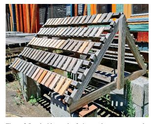
**Figure 2** Stand with samples facing south at exposure angle of 45°
