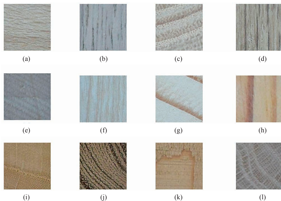
Figure 1 Images display samples of twelve wood species. (a) European Beech, (b) Common Walnut, (c) Sweet Chestnut, (d) Turkey Oak, (e) Common Alder, (f) Manna Ash, (g) Norway Spruce, (h) Scots Pine, (i) Tree of Heaven, (j) Black Locust, (k) Mediterranean Cypress, (l) Oriental Plane
