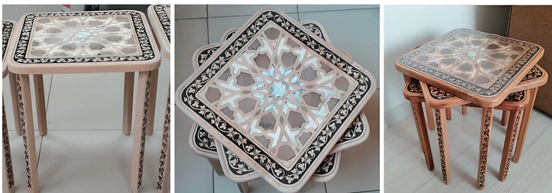
Figure 5 a) Assembled coffee table, b) sanded version of tables, c) varnished version of integrated tables
