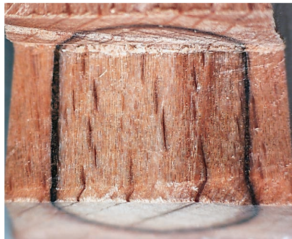
Figure 3 Sections of welded unmodified dowel into unmodified base; tip of the dowel is turned upwards (Župčić, 2010)
