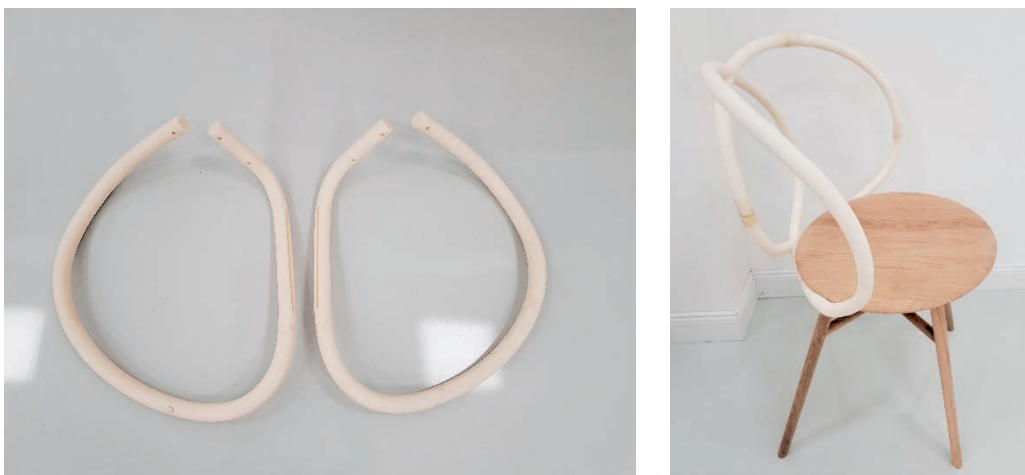
Figure 6 Example of backrest product development (rapid prototyping) in Croatian furniture manufacturing; (Jarža, L., photography, 2022)
