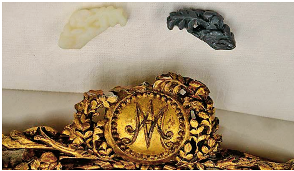
Figure 4 3D printed element created by reverse engineering ( https://3dprint.com/45399/marie-antoinette-museum-chair/ ) Slika 4. 3D printani elementi kreirani povratnim inženjeringom ( https://3dprint.com/45399/marie-antoinette-museum-chair/ )
