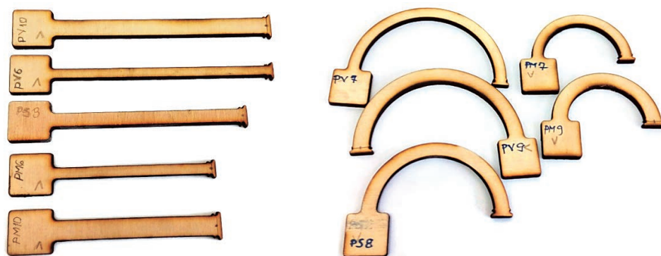
Figure 4 P-type specimens: a) straight cantilever, b) half-circle cantilever
