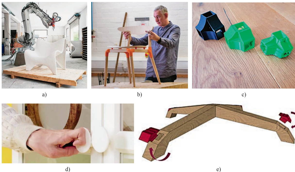
Figure 3 Uses of 3D printing in production: a) 3D printed large scale chair ( https://parametrichouse.com/3d-printed-furniture/ ); b) Part of furniture ( https://ultimaker.com/learn/3d-printing-in-furniture-design ); c) Joints development (Prekrat, S., photography); d) Parts for testing of ergonomics ( https://3dprinting.com/3d-printing-use-cases/how-the-furniture-industry-benefits-from-3d-printing/ ); e) Replacement of parts (Jarža, L., photo of rendered 3D model)
