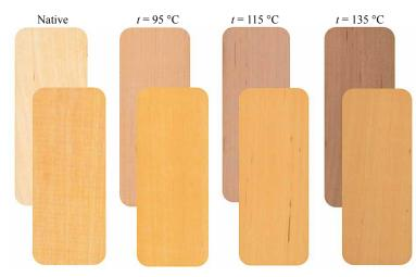
**Figure 2** View of alder wood before and after UV irradiation: native; steamed at t = 95 °C; steamed at t = 115 °C and steamed at t = 135 °C
