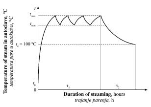
Figure 1 Mode of colour modification of alder wood with a saturated steam-air mixture or saturated water steam Slika 1. Način promjene boje drva johe smjesom zasićene pare i zraka ili zasićenom vodenom parom
