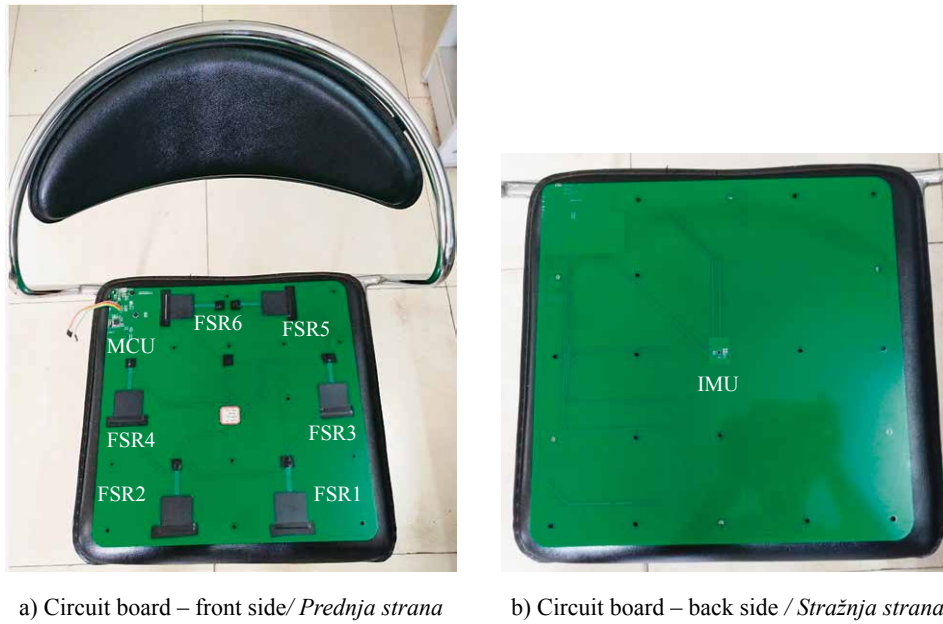
Figure 4 Smart cushion circuit board on a chair (Ma et al. , 2017)
