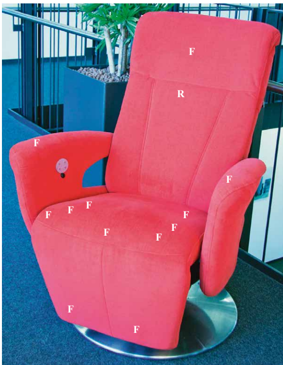
Figure 9 Smart chair with integrated sensors locations (F – FSR, R – radar) (Hesse et al. , 2017) Slika 9. Pametna stolica s rasporedom integriranih senzora (Hesse et al. , 2017.)
