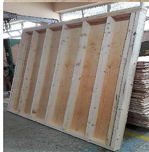
Figure 1 Standard wood frame (ASTM E 72, 2014) and shear wall sheathing with plywood
