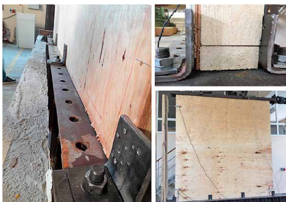
Figure 3 Mounting of shear wall to floor
