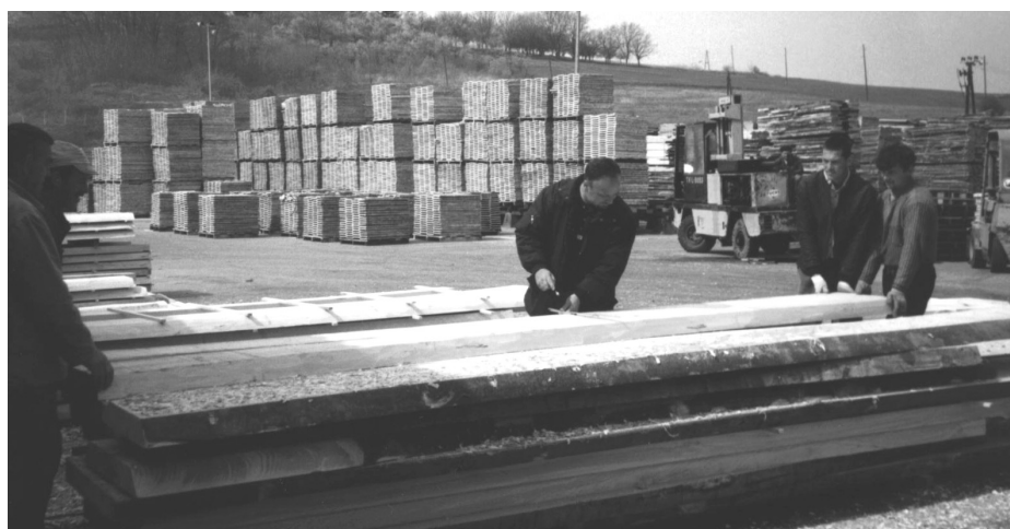
Slika 1. Preuzimanje bukovich samica i polusamica Figure 1 Handling of the unedged and half-edged beech boards
