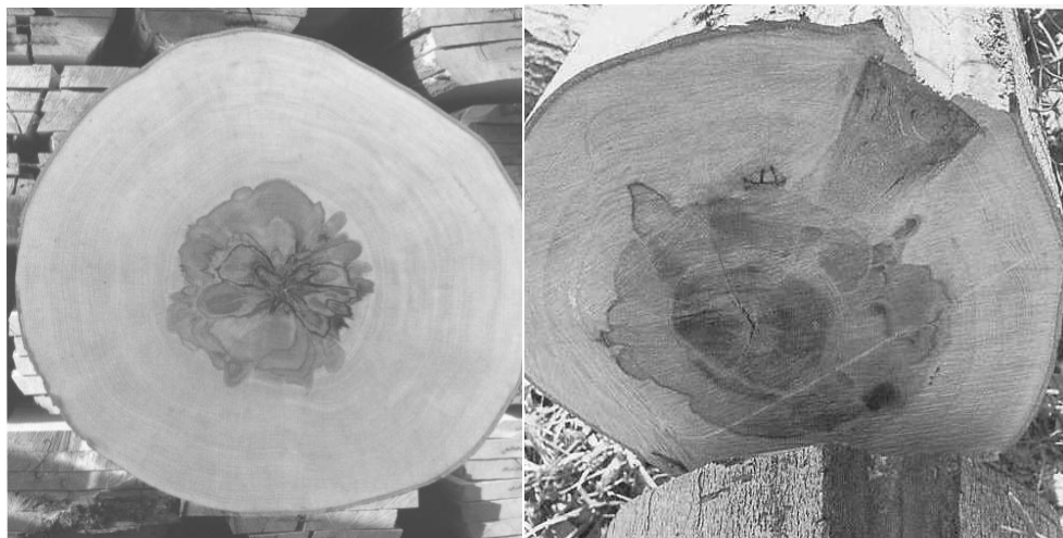
Slika 1. Neprava srž u bukovu trupcu Figure 1 (Red heart rot) False heartwood in a beech (tree stem) log
