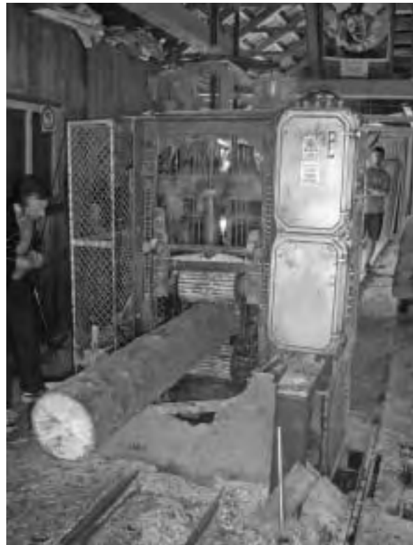
Figure 10 Small frame saw (photo by author) Slika 10. Mala pila jarmača (foto: Bomba)
