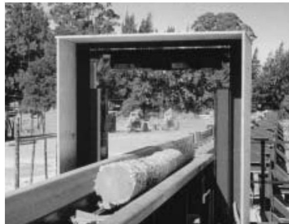
Figure 2 A measuring device identical with the device installed in the Stará Ves sawmill where a substantial part of measurements was carried out (a scanning frame with a vertical and horizontal system placed in front of the log sorter)
