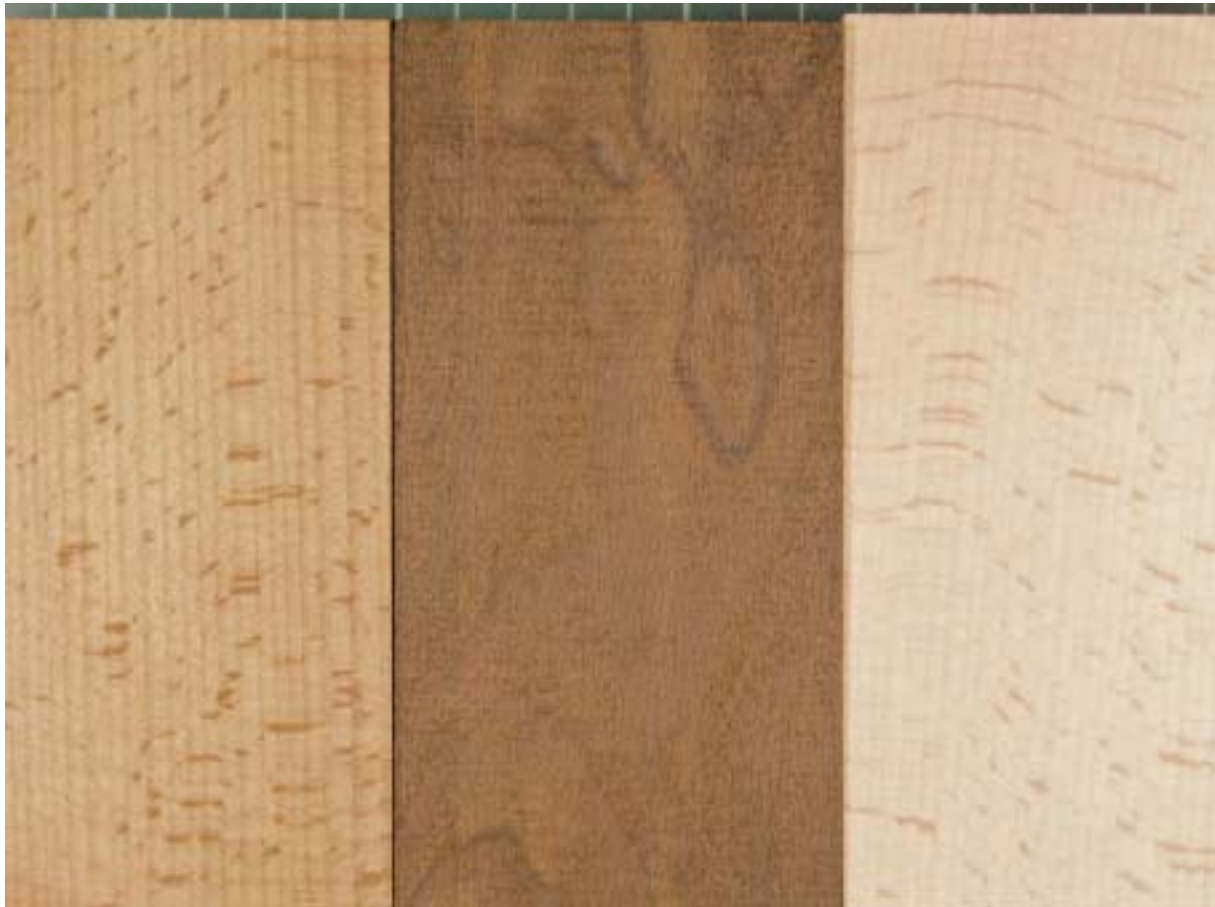
Slika 1. Prirodna bukovina (desno) i toplinski obrađena bukovina pri različitim temperaturama (lijevo i u sredini); foto: Turkulin Figure 1 Genuine beech-wood (right) and heat-modified wood treated at various temperatures (left and middle). Photo: Turkulin
