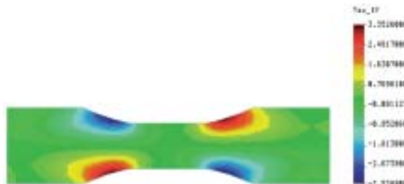
Slika 9. \tau_{xy} naprezanje u okomitom sloju Figure 9 \tau_{xy} stress in perpendicular layer
