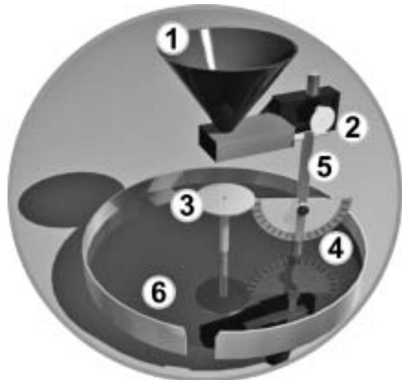
Figure 5 Langhaus equipment for measuring bulk angle 1 – loading hopper, 2 – screw for height adjustment, 3 – circular plate ø 50 mm, 4 – angle gauge, 5 – measuring rod, 6 – collecting vessel
