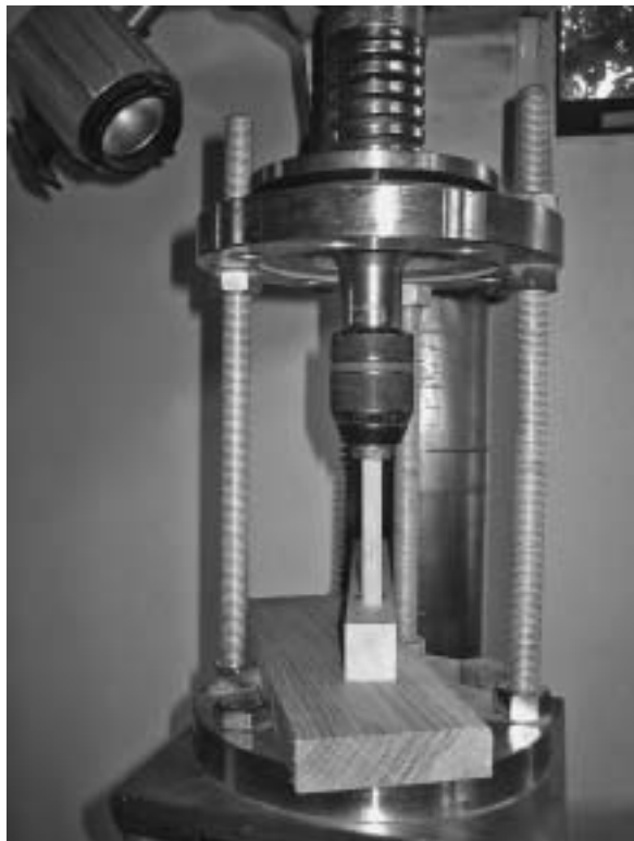
Slika 4. Zavarivanje moždanika za podlogu Figure 4 Welding of dowels into the basis
