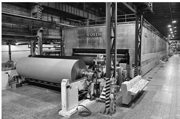
Figure 1 Semi chemical fluting reel at the end of a paper machine Slika 1. Namotavač polukemijskog fluting papira na kraju papir-stroja
