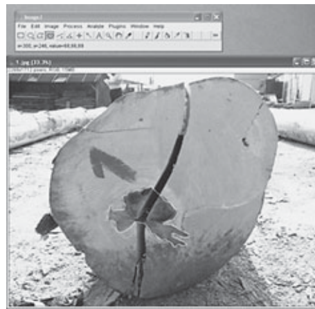
Figure 2 Analysis of false heartwood by software product ImageJ
