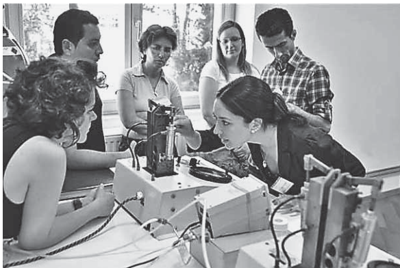
Figure 5 Microtensile strength testing on Pulmac testing device
