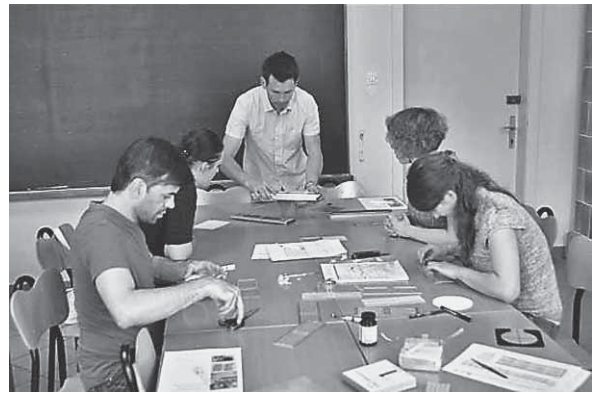
Figure 4 Preparation of thin wood strips for accelerated exposure in QUV device
