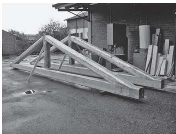
Figure 1 Uso Fiume larch beams are traditionally used by the Aosta Valley sawmilling industry for producing wooden carpentry
