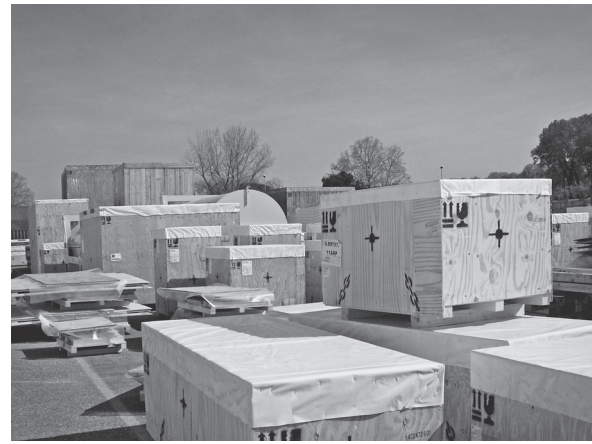
Figure 4 A heavy load industrial wood packaging (about 90 tons of payload) produced according to UNI 9151 before closing of the case (left); industrial wood packaging ready for shipment (right)
