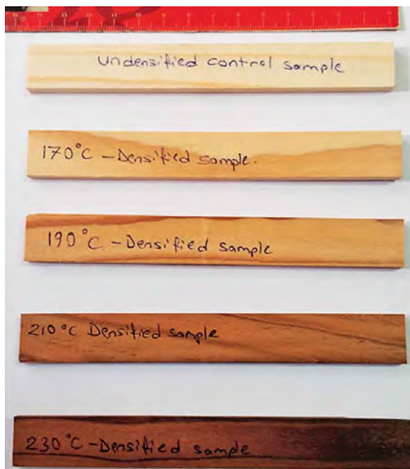
Figure 1 Undensified control specimen and heat-treated/densified specimens
