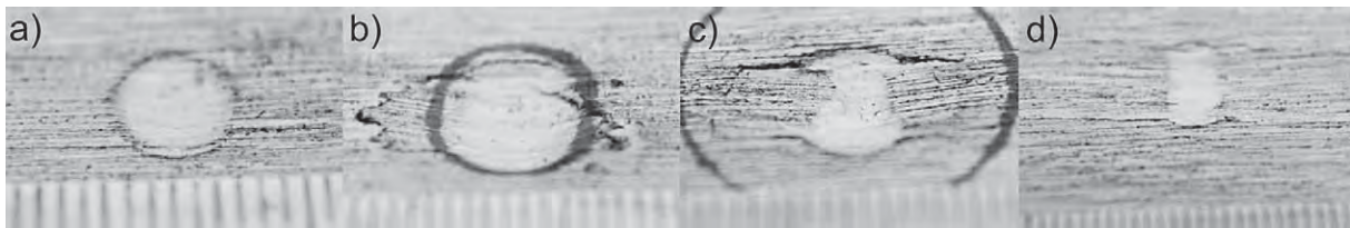
Figure 3 Sample indentations in the surface of layered composite samples with round gaps simulating knotholes located in layer 2 (variant I) after hardness testing: a) control sample, b) sample with a 10 mm round gap, c) sample with a 20 mm round gap, d) sample with a 50 mm round gap
