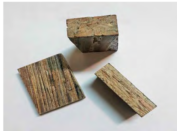
Figure 3 Examples of test specimens from date palm rachis-based LSL blocks
