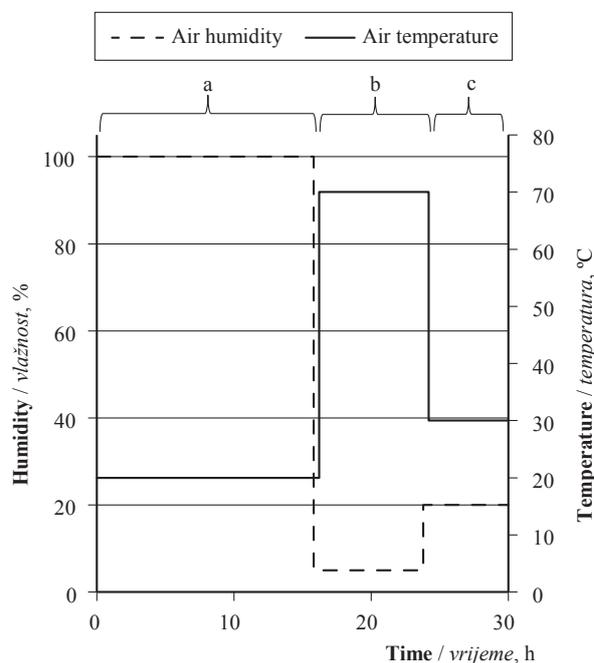
**Figure 2** Changes in humidity and temperature during a full cycle of artificial weathering: a) soaking in water for 16 hours, b) drying at 70° C for 8 h, c) UV irradiation for 6 hours
