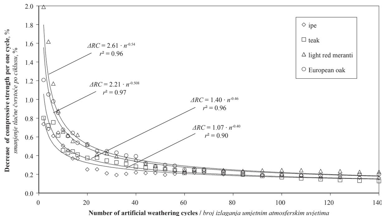
**Figure 3** The dependence of decrease of compressive strength along fibers after one cycle of artificial weathering on the number cycles of artificial weathering for light red meranti, ipe, teak and European oak
